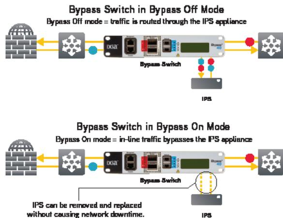
By logging into the device from anywhere on the network, operators can monitor traffic and device status, and configure and control the device. One aspect of device control is the ability to force the bypass switch into Bypass On mode, taking the IPS offline. This capability can be handy for easily removing the IPS from service without requiring a technician to be physically on site with the IPS, saving time and travel costs.
