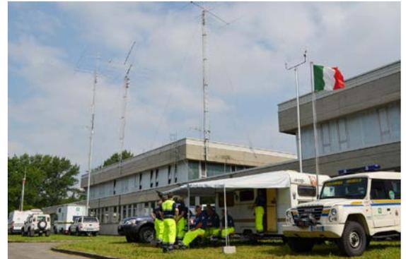
**Figure 3: The close proximity of different radio services means that intermodulation can be expected.**
