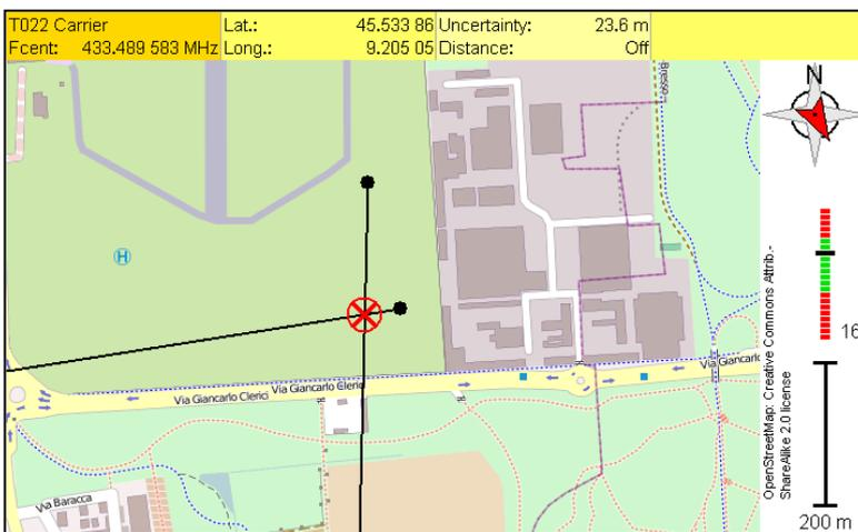
**Figure 6: Taking cross bearings on the emitter on channel T022 locates the source of interference.**
